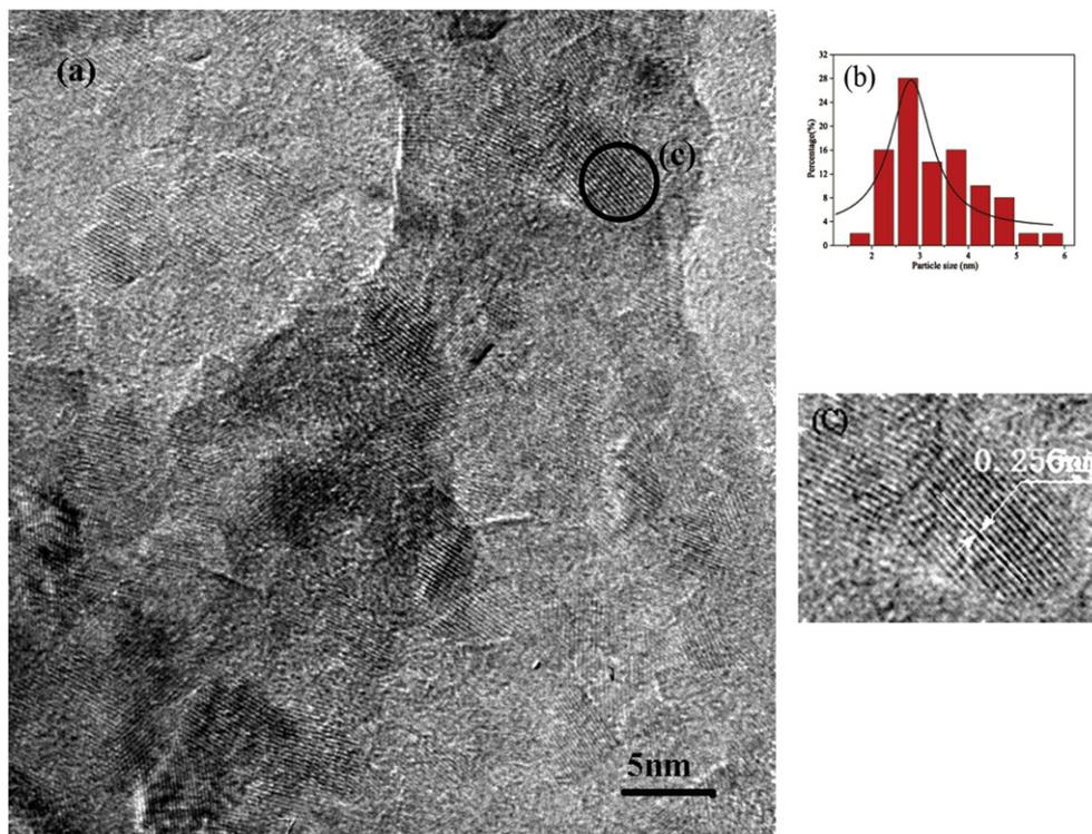
Fig. 1. (a) TEM image of the GQDs, (b) the corresponding size distribution, and (c) high-resolution TEM image of single GQD.
