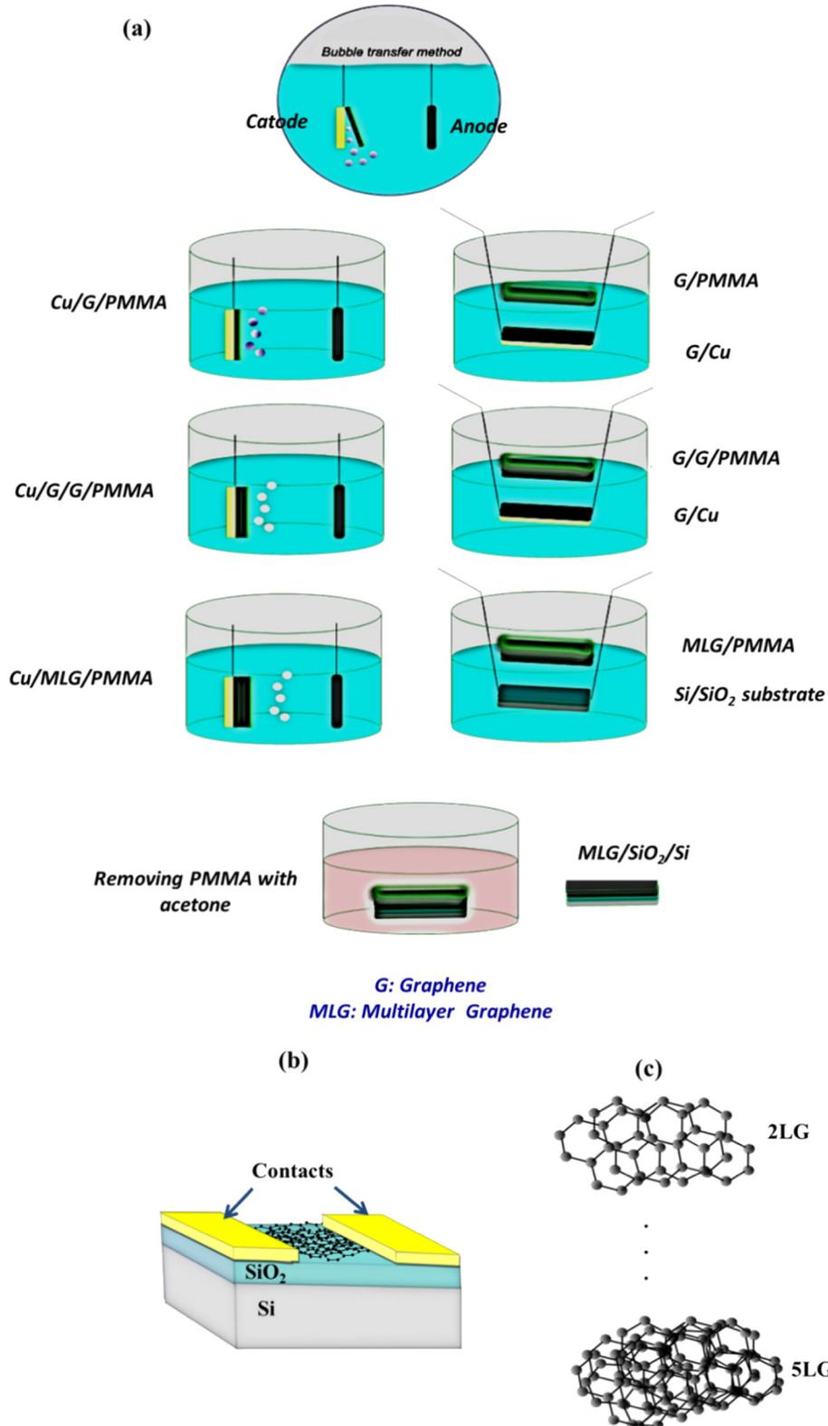
Fig. 1. (a) Consecutive bubble transfer method; (b) device schematic; (c) transferred turbostratic structure.
