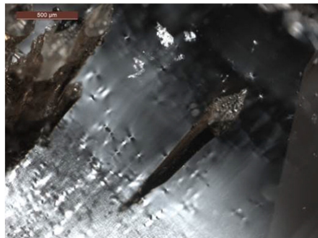
Fig. 3. Photomicrograph of a channel under crossed (linear) polarizers of sample MSC67. There is less to no abnormal birefringence next to the channels, while the rest of the diamond is strained (especially around the disk-crack-like defects).
