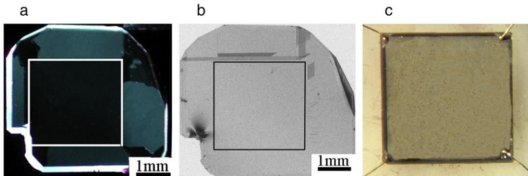
**Fig. 1.** Photoluminescence (a), and X-ray topography (b) maps of diamond plate cutting schemes for making rectangular homogeneous sample without extended defects for Hall effect measurements (c).
