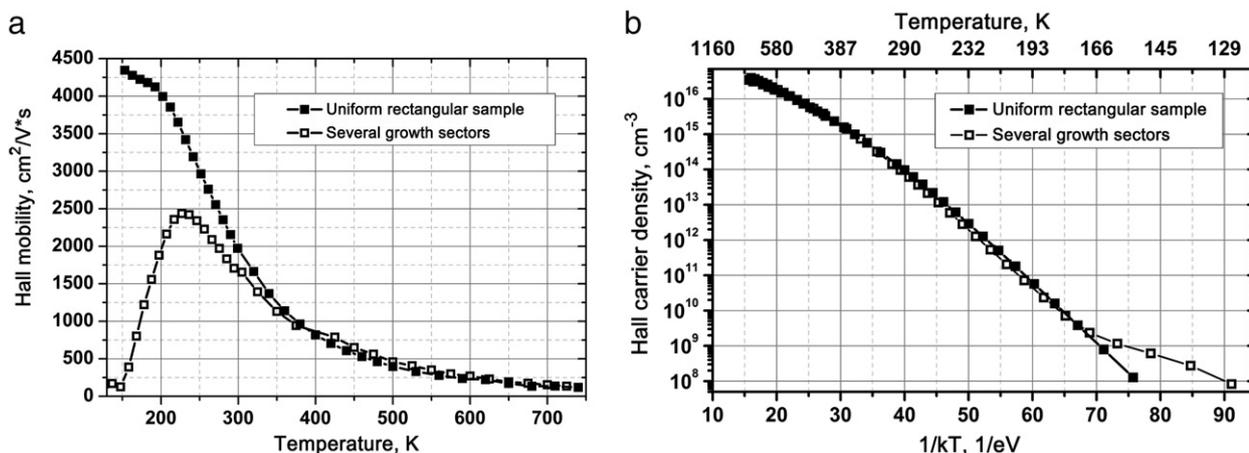
**Fig. 2.** Hall mobility (a) and the density of holes (b) temperature dependencies measured on unshaped (empty squares) and rectangular cut diamond plates without extended defects (full squares).
