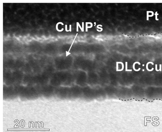
**Fig. 1.** Typical TEM cross-section micrograph of DLC:Cu film illustrating structure of the DLC:Cu film (Cu nanoparticles embedded into the DLC matrix). FS stands for fused silica substrate, Pt – platinum used for sample preparation. The arrow indicates Cu nanoparticle. Scale bar length is 20 nm. Investigated film contains  $\sim 33$  at.% Cu.
