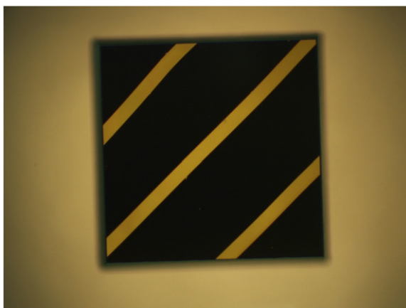
Fig. 1. Single crystal diamond with diagonal graphitic implant. Yellow region is unimplanted region and the dark region is ion implanted region. Sample is approximately 3 mm×3 mm in area.
