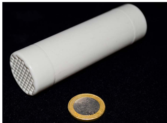
Fig. 1. Ceramic membrane monolith comprising 55 feed channels.
