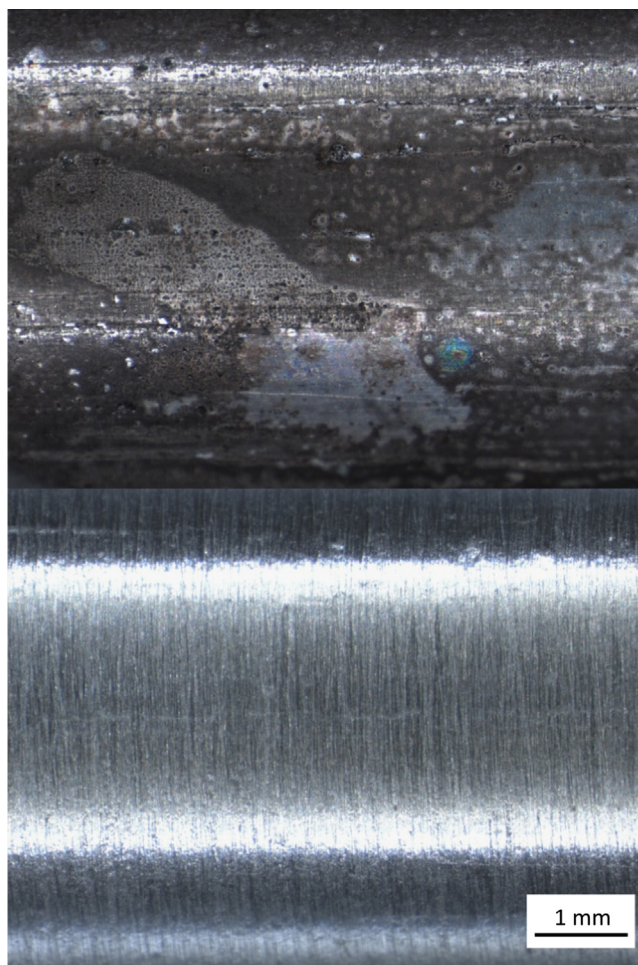
Fig. 1. Macrograph of vanadium tube surface as received (top) and after cleaning (bottom).
