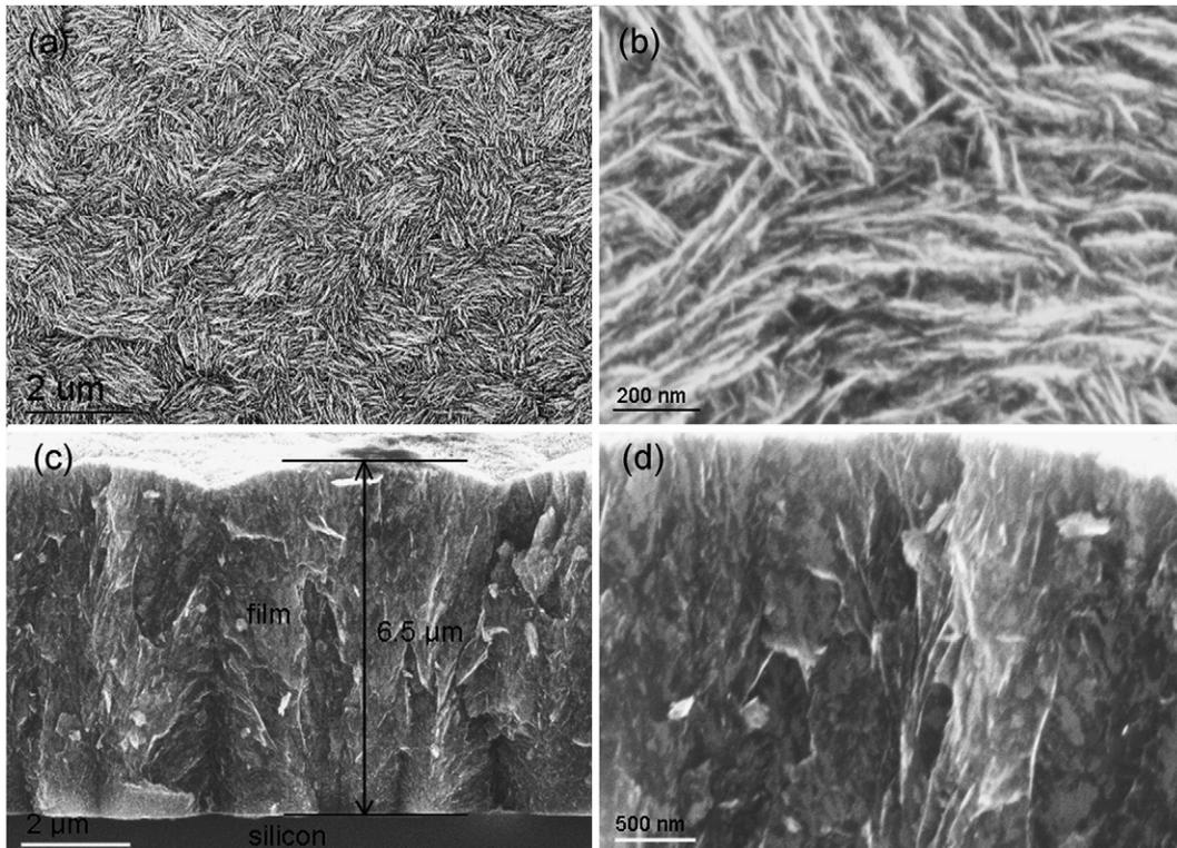
Fig. 1. Plane view SEM images of high density elongated nanocrystallites revealing the rod-like morphology (a) at low magnification and (b) at high magnification. SEM images of a cross section (c) indicate the thickness of  $\sim 6.5$   $\mu\text{m}$  after 2 h of deposition and (d) high magnification highlighting the many embedded nanorods in the film.
