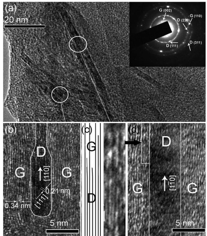
Fig. 2. (a) Low magnification TEM image indicating numerous nanorods. The inset shows the corresponding SAED pattern. The different diamond (D) and graphite (G) rings are indicated; (b, d) HRTEM images of diamond nanorods with an average d-spacing of 0.21 nm surrounded by  $\sim 5$  nm thick graphite sheets with d-spacing of 0.34 nm. (c) Schematic indicating the lattice spacing of graphite and diamond structures.
