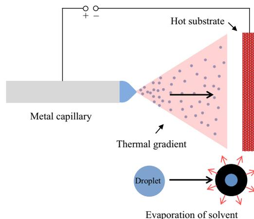
Fig. 1. Schematic diagram of electrospinning deposition for synthesizing ZIF-7 membranes.
