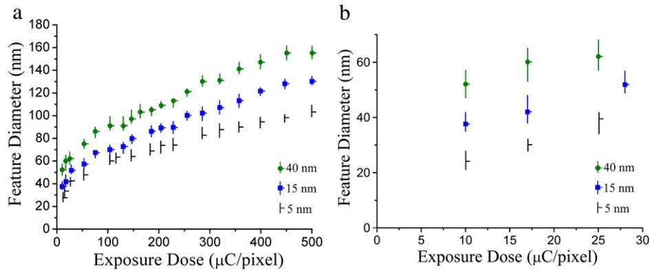
**Fig. 1.** (a) A comparison plot of feature diameter (nm) against dose (μC/pixel) for three samples containing an Al CDL on PMMA on diamond. The bottom contour is the 5 nm thick version, the middle one 15 nm and the top contour 40 nm. (b) An expansion of the first 30 μC/pixel results. The vertical lines for all plots represent error bars covering 8 measurements per inspected dose.
