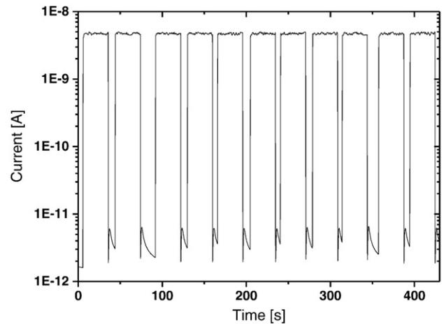
**Fig. 1.** The current signal of the SCDD registered for 100 MU with a dose rate of  $200 \text{ MU min}^{-1}$ .
