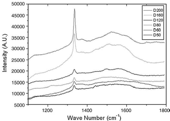
**Fig. 1.** Raman spectra of polycrystalline CVD diamond films according to the deposition time.
