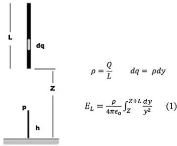
Fig. 1. Electric field  $E_L$  at  $P$ , caused by a downward leader of length  $L$  and linear charge distribution  $\rho$ .
