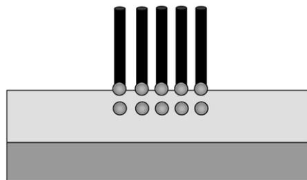
It is well known that the higher the dose amount, the larger the sputtered depth [14]. Sputtered depths measured by atomic force microscopy (AFM) after ion implantation were in agreement with this tendency. As a result, the Ni concentration at the surface increased with increasing the dose.
