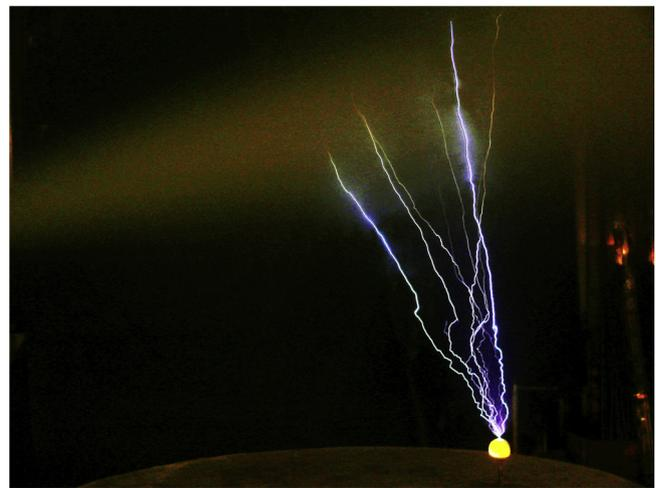
**Fig. 3.** Discharge development in a cloud of charged water aerosol and in the gap between lower artificial charged cloud and ground.
