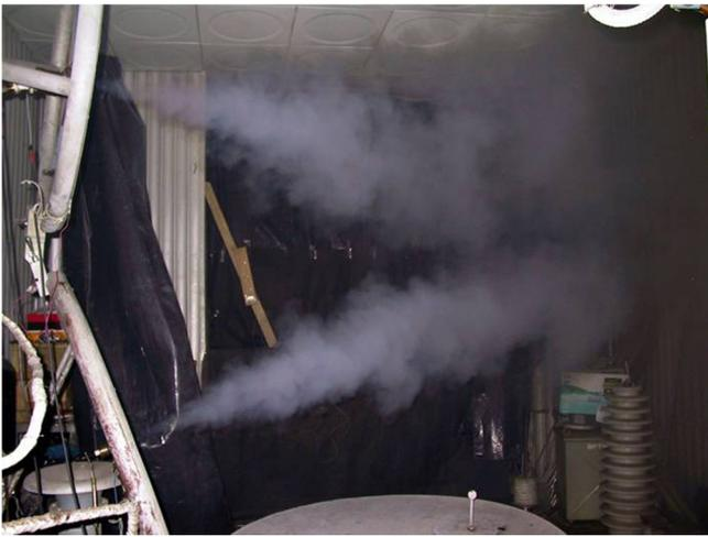
**Fig. 1.** Picture of disposition of artificial charged clouds in aerosol chamber: outlet current of charged aerosol generator for upper cloud –  $100 \mu\text{A}$ , for lower cloud –  $110 \mu\text{A}$ .
