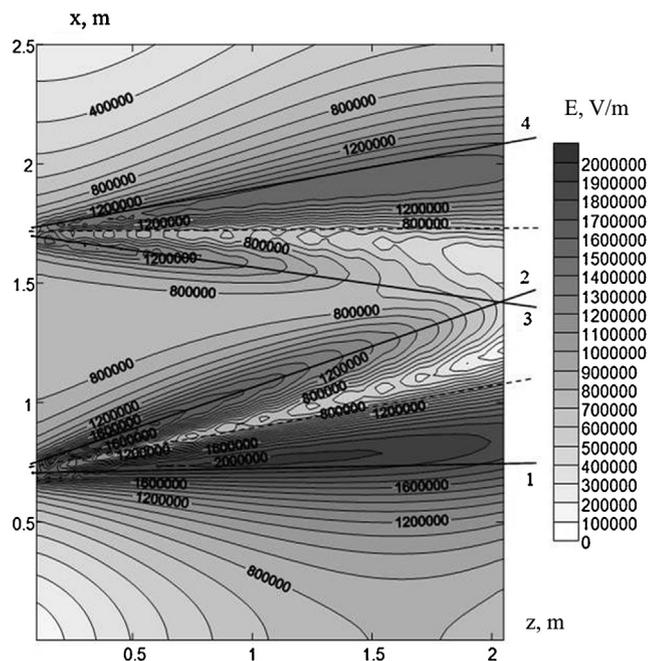
**Fig. 2.** Distribution of electric field strength in a vertical section of the gap “two vertically separated clouds – grounded plate”: 1 and 2 – boundaries of the lower artificial charged aerosol cloud; 3 and 4 – boundaries of the upper artificial charged cloud.
