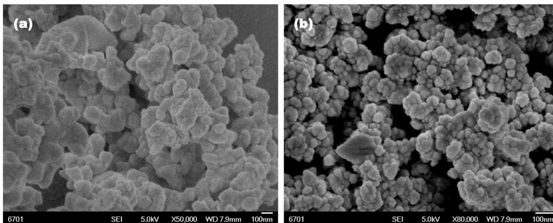
Fig. 1. SEM image of BiFeO<sub>3</sub> (a) and Co/BiFeO<sub>3</sub> (b) nanoparticles.
