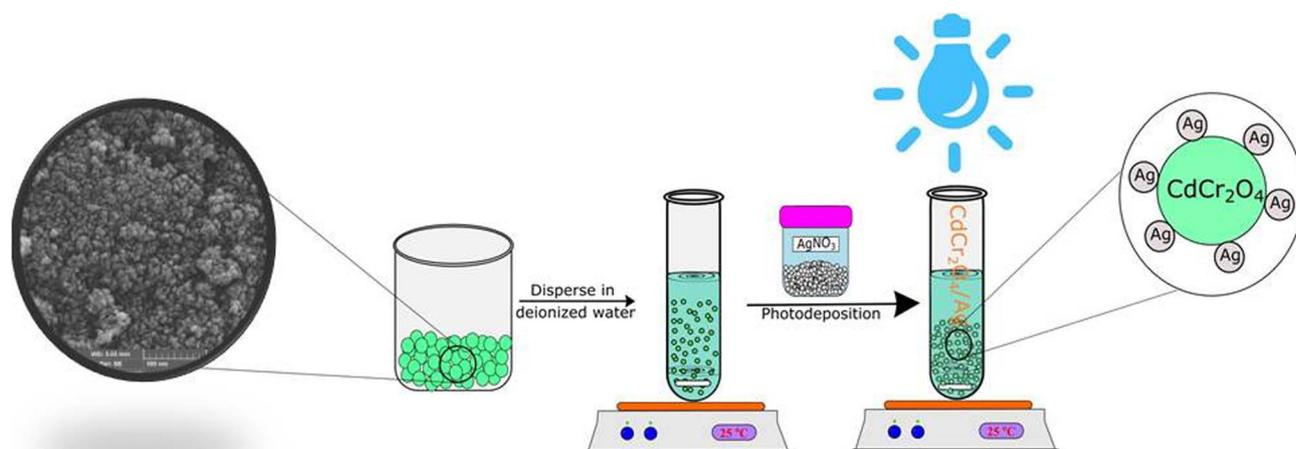
**Scheme 1.** Schematic diagram of the synthesis of CdCr<sub>2</sub>O<sub>4</sub>/Ag nanostructures.
