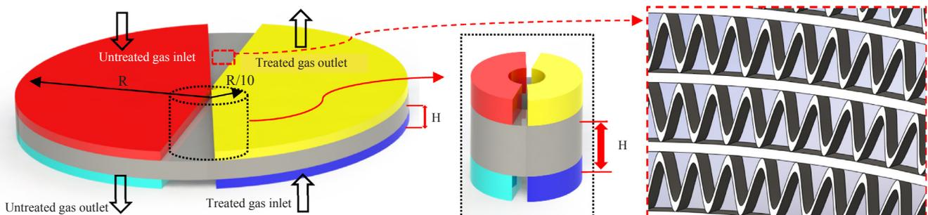
Fig. 1. Corrugated sinusoidal ducts.
