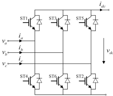
Fig. 1. Schematic diagram of the three-phase two-level VSC.
