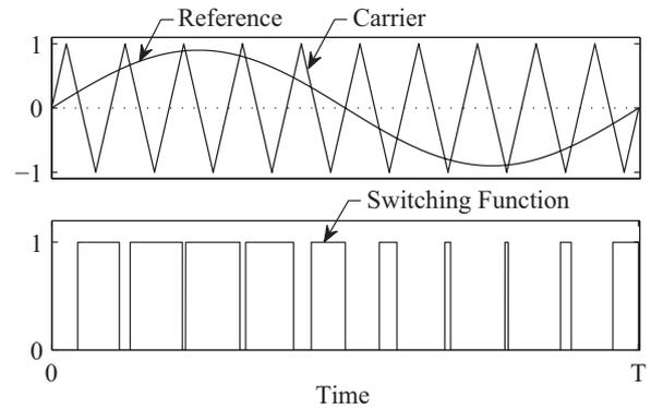
Fig. 2. NSPWM process of ST1 ( $m_f = 10$ ).
