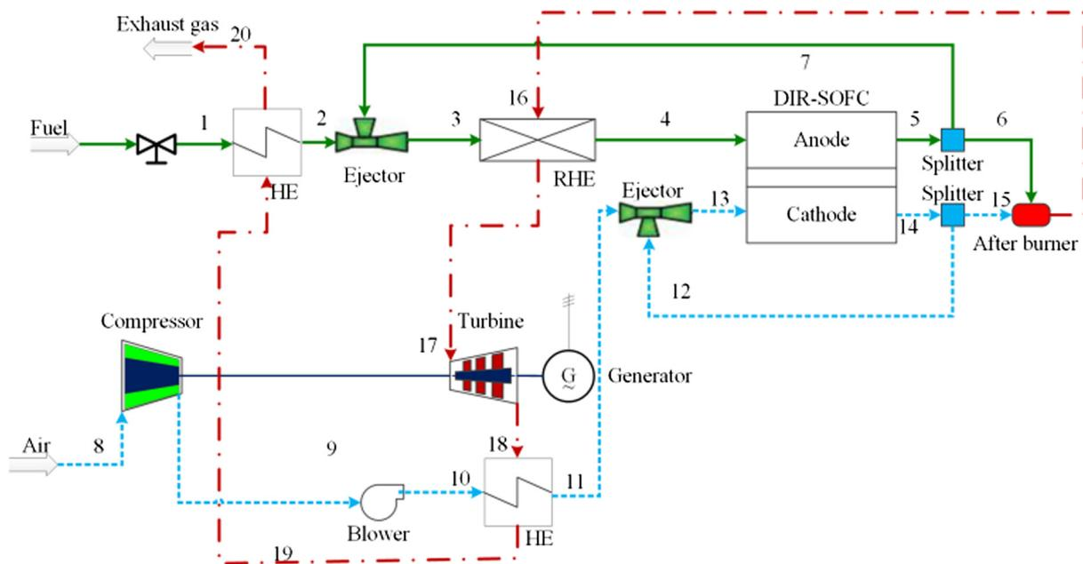
Fig. 1. The integration scheme of the SOFC-GT system.
