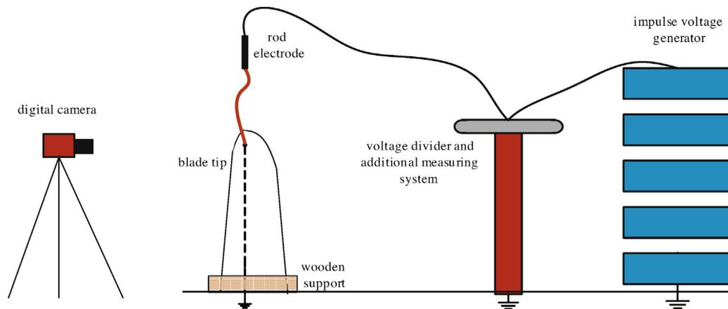
Fig. 1. Experimental test system.
