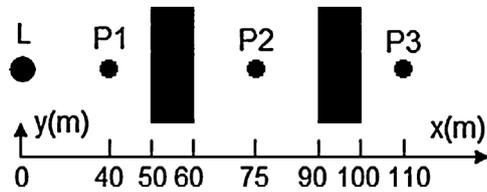
Fig. 1. Top view of the system analyzed. Black rectangles: buildings; L: lightning; P1, P2, P3: field measurement points.
