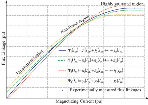
Fig. 1. Different configurations to represent saturation characteristics of a typical electrical machine.
