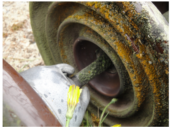
Fig. 1. Biological soiling of insulator in Balsillas.
