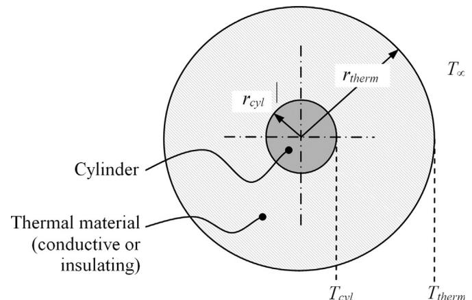
Fig. 1. Cylindrical heat transfer system.
