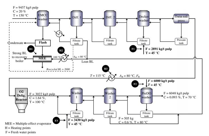
Fig. 1. Base case simulation model for an existing BSWS (symbols F, C and T represent the flowrate, DS concentration and temperature, respectively).
