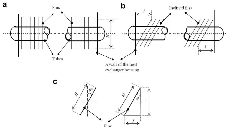
Fig. 1. Representation of the influence of the inclination angle of fins on their number; (a) fins and tube perpendicular to each other, (b) heat exchanger with inclined fins, (c) representation of the tube part, which cannot be covered with fins.
