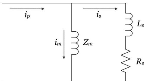
Fig. 1. Simplified equivalent circuit of a CT.
