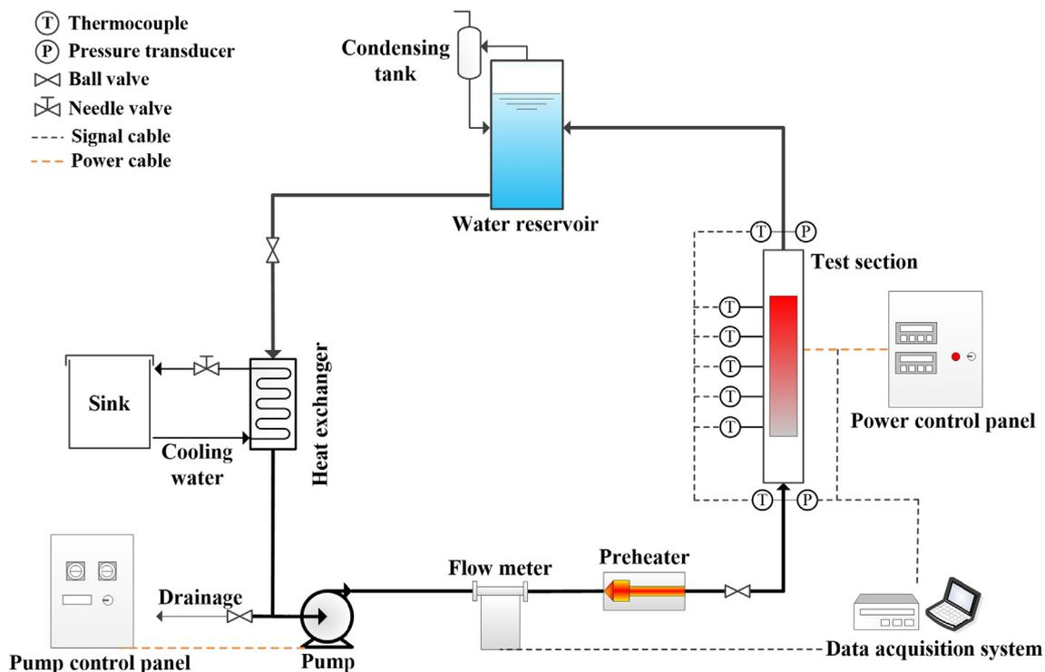
Fig. 1. Schematic drawing of the experimental loop.
