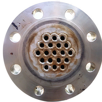
Fig. 3. Regular triangle arrangement of tube bundle.
