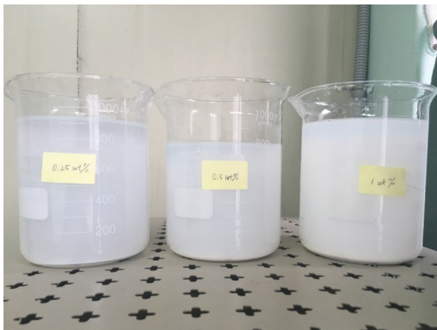
Fig. 1. Photograph of \text{Al}_2\text{O}_3 nanofluids (0.25 wt%, 0.5 wt%, and 1.0 wt%).
