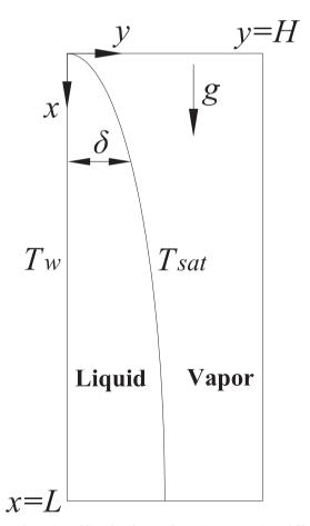
Fig. 1. Configuration of liquid and vapor layers in computation of film condensation.
