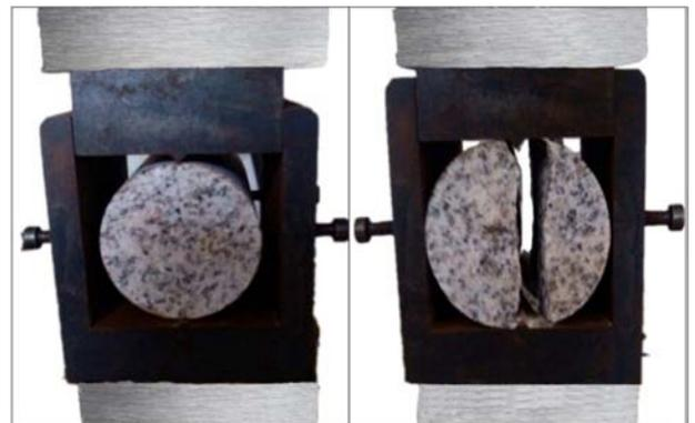
Fig. 1. The cylindrical rock before and after the Brazilian split.
