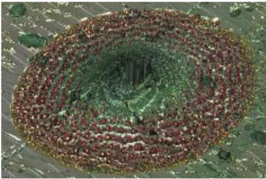
Fig. 2. Micromorphology of a laser-ablated Si APD.
