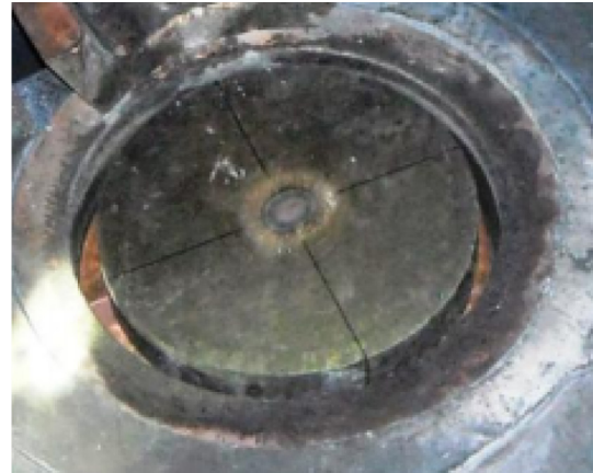
Fig. 1. Test block sitting at the top of the mould in the plasma arc furnace.
