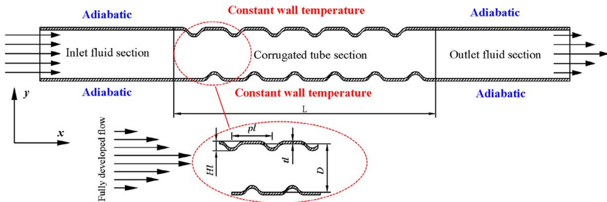
**Fig. 1.** Schematic diagram of the computational domain.
