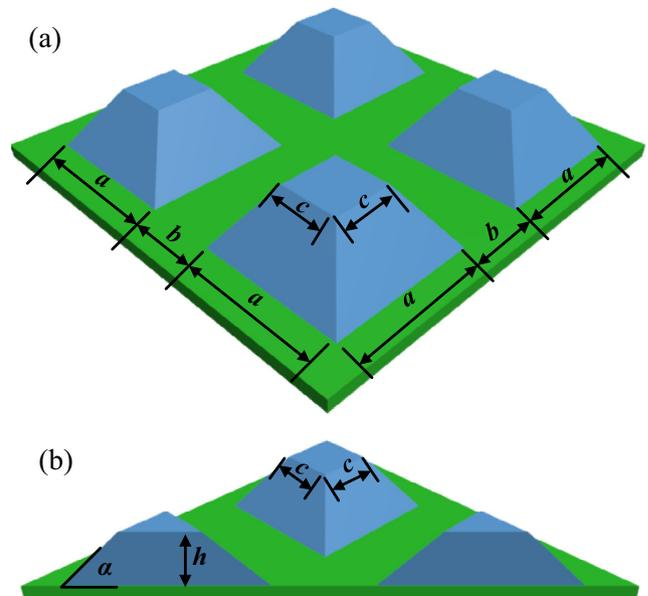
Fig. 1. Definition of the trapezoidal microarchitecture.
