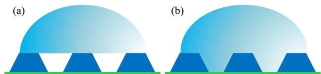
Fig. 2. Two wetting states of a droplet on a microarchitected solid surface. (a) Composite state. (b) Non-composite state.
