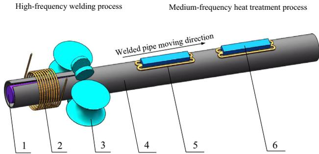
**Fig. 1.** Schematic of HFIW pipe production process. (1) Magnetic rod (2) high-frequency induction coil (3) squeezing rollers (4) welded pipe (5) medium-frequency induction coil (6) magnetic conductor.
