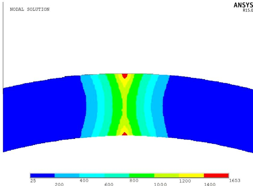
**Fig. 2.** The “sandglass” shaped temperature field of high-frequency welding.
