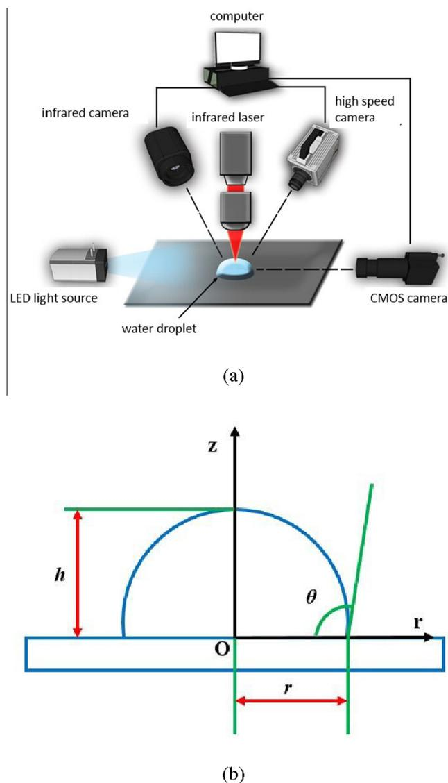
Fig. 1. (a) Schematic of the experimental setup system and (b) illustration of the droplet profile.
