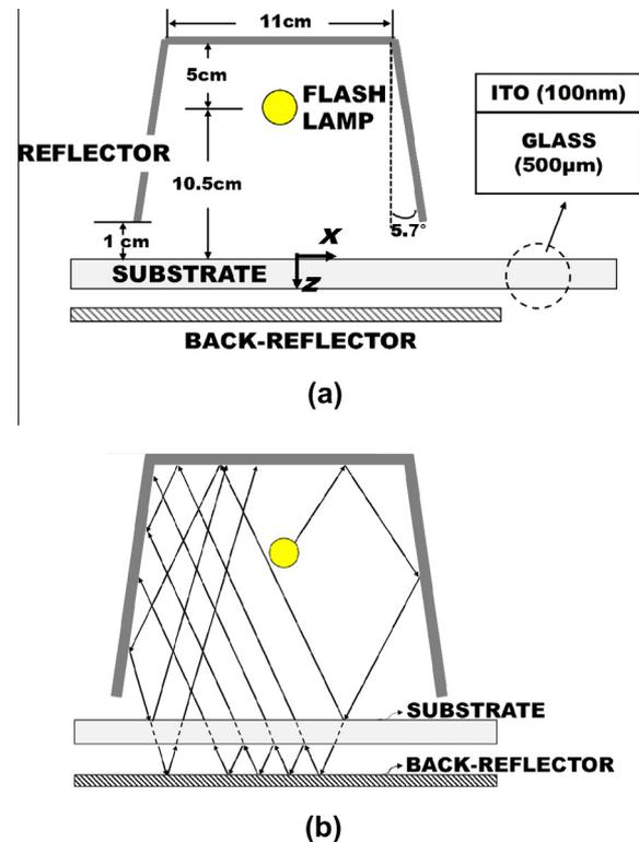
Fig. 1. (a) Flash lamp annealing (FLA) system for the ITO thin-film deposited on glass substrate and (b) tracing of light emitted from the lamp.
