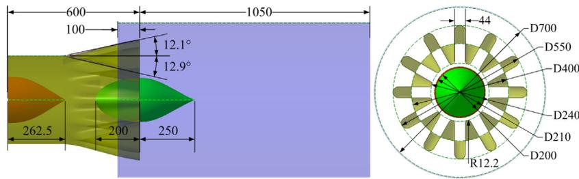
Fig. 1. Geometrical dimensions of the plugged-lobe mixer.
