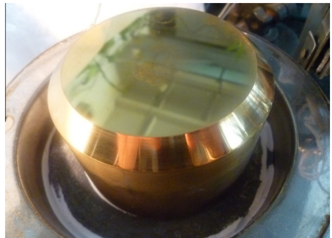
Fig. 1. The working section with mirrored gold-plated surface.
