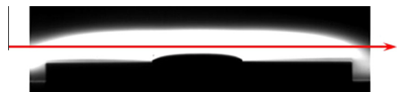
Fig. 1. Schlieren image of the vapor cloud surrounding a pinned, sessile hexane drop. The bright region indicates the presence of vapor and the arrow demonstrates a path of the infrared beam from the FTIR through the vapor cloud.
