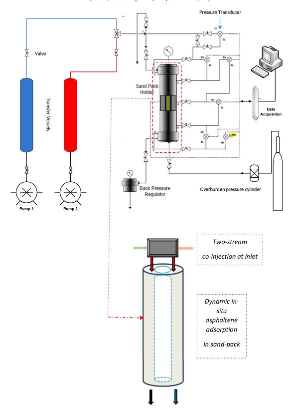
Fig. 1. Experimental rig designed for dynamic flooding.
