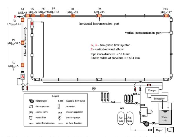
Fig. 1. Simplified schematic diagram of the test facility (not to the scale). For the current experiments, injector A is used as the inlet and injector B is used as the exit.
