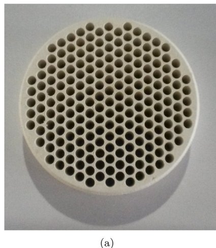
Fig. 1. Geometry used in the model. (a) Photograph of the porous media, (b) computational reconstruction of the porous media.
