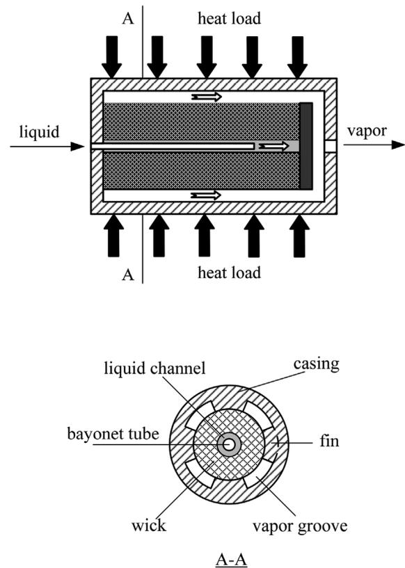
Fig. 1. Sketch diagram of porous wick evaporator with bayonet tube.
