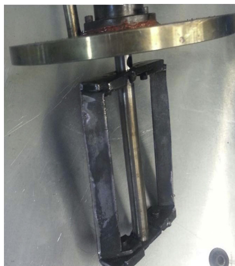
Fig. 1. Vertical blade stirrer (vertical length = 0.11 m, thickness = 0.0025 m).
