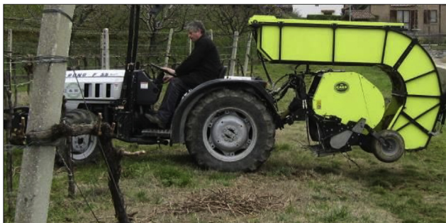
Fig. 1. The harvest machinery combination composed of a narrow-track tractor, a small diameter round baler and a baler accumulator.
