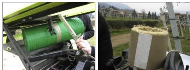
Fig. 2. The baler was used, alternatively, with a plastic net tying system (left) or a twine knotter based on natural twine (sisal; right), in order to obtain bales secured with materials eventually compatible with direct burn-up.
