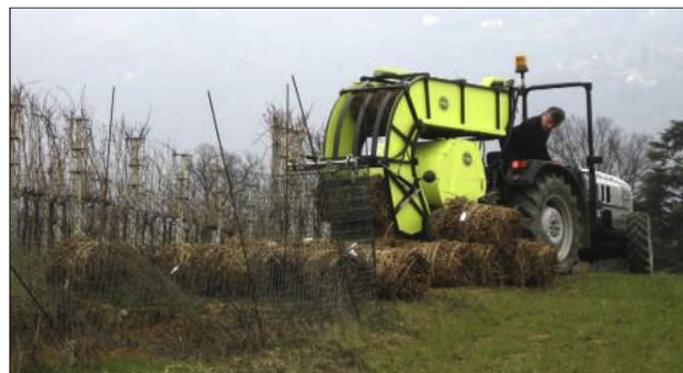
Fig. 3. The bales' accumulator is able to unload automatically the 7 bales stored into the tunnel, while the bale contained into the baler chamber is discharged at the end of this operation, independently.
